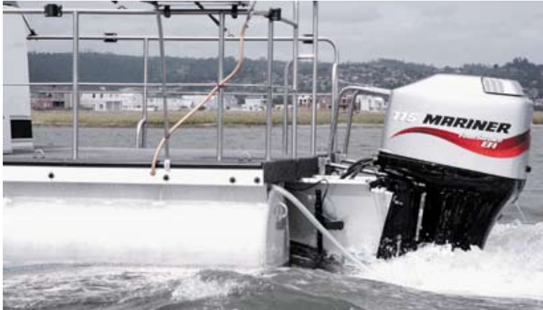
A 115 HP outboard is a little over the top for a cruising craft . A 60HP Mercury Big Foot is ideal.
